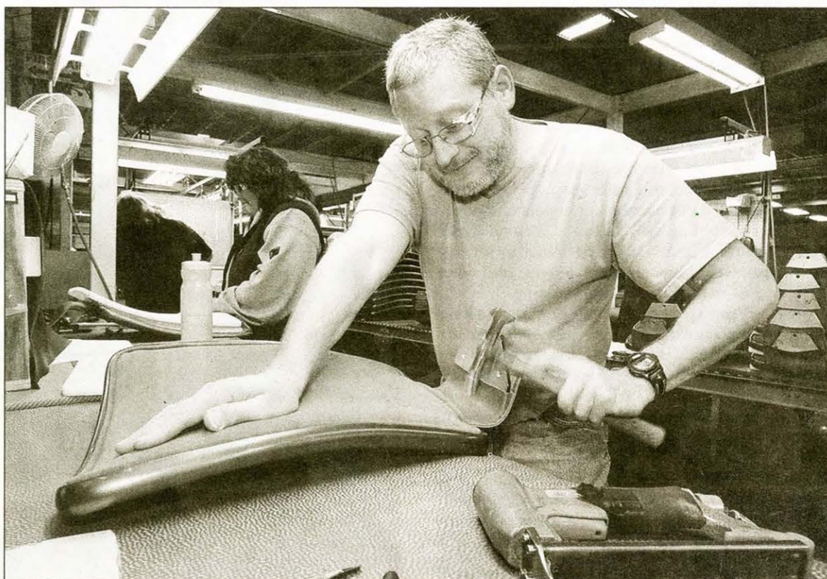
David Ghizzoni applies upholstery to a chair back. Gasser Chair developed the vinyl trim exclusively for its products.
